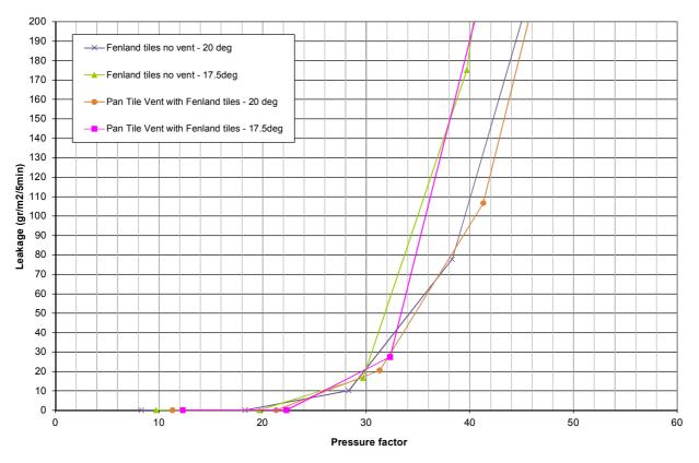
Figure 4 Pressure factor v leakage curves for the Fenland tiles and Manthorpe Pan Tile Vent
