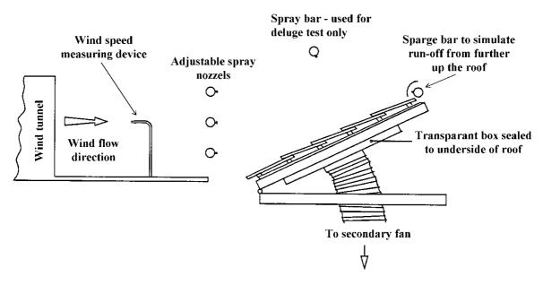
Figure 3 Schematic view of the BRE Rain Penetration Test Rig
